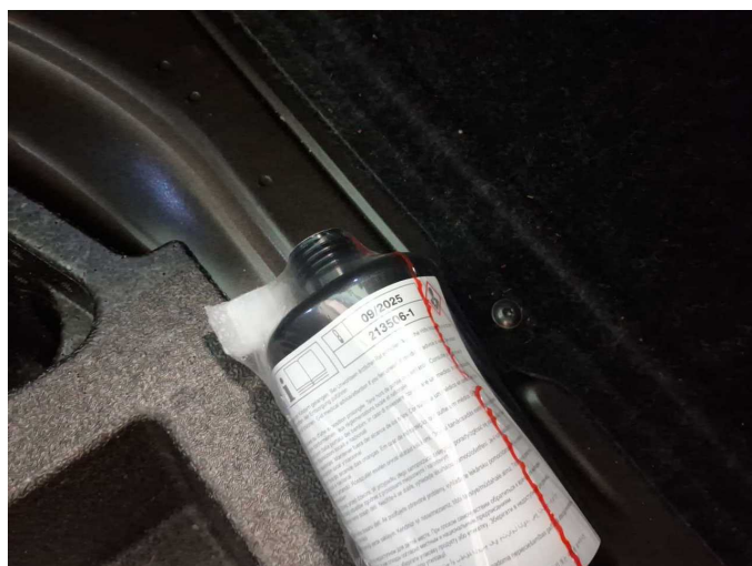
Damage 2: Equipment: Tirefit filler - Expired - Replace
