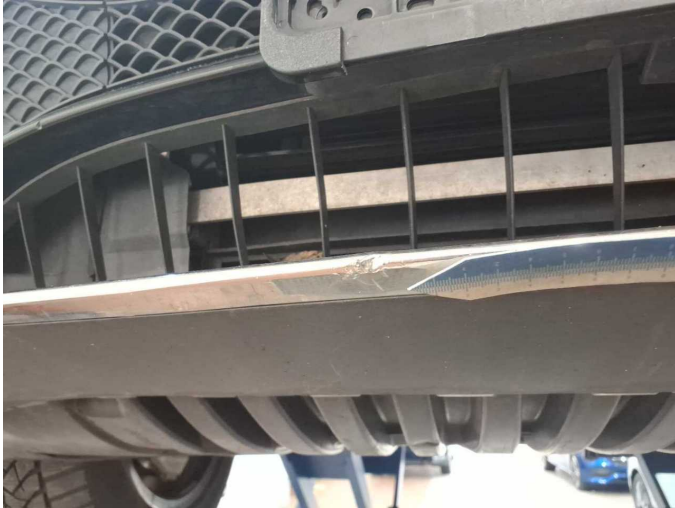
Damage 5: Front bumper: Spoiler (Lippe) - dent(s) - Replace
