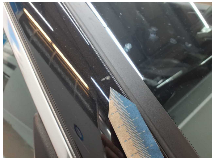
Damage 6: Body: B-pillar - right side - Scratch(es) - Smart repair
