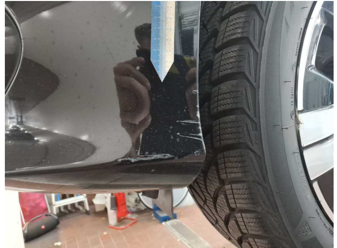
Damage 10: Front bumper: Front bumper - Dent / paintcoat damage - Repair and paint
