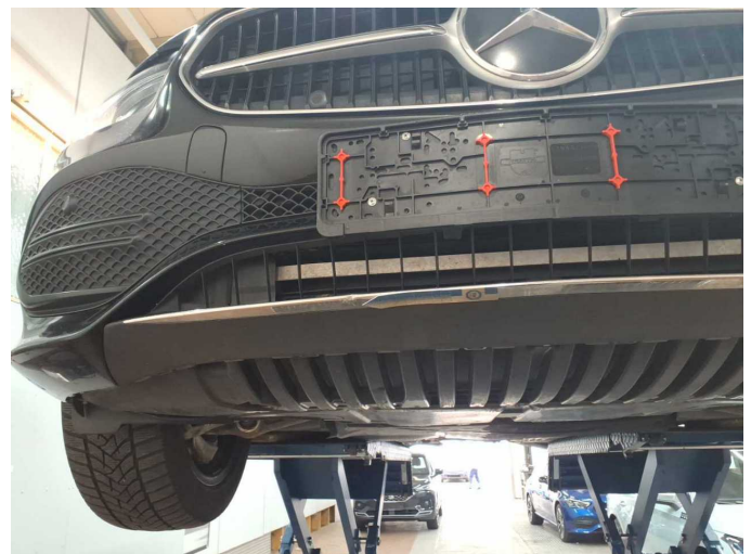
Damage 5: Front bumper: Spoiler (Lippe) - dent(s) - Replace
