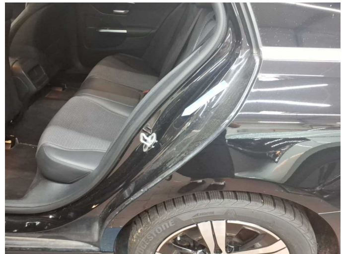
Damage 4: Side panel - rear left side: Sill - dent(s) - Smart repair
