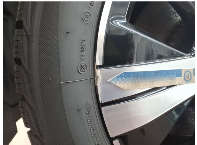
Damage 8: Wheel / tyres: Alloy rim - front left side - Scratch(es) - Loss in value
