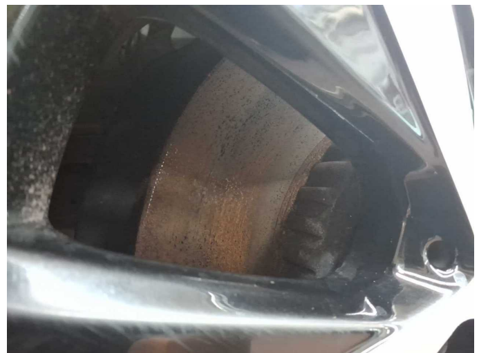
Damage 7: Braking system: Brake discs - front (Und hinten / freibremsen) - Corrosion
