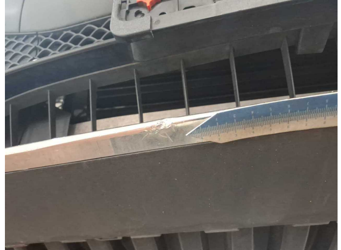
Damage 5: Front bumper: Spoiler (Lippe) - dent(s) - Replace
