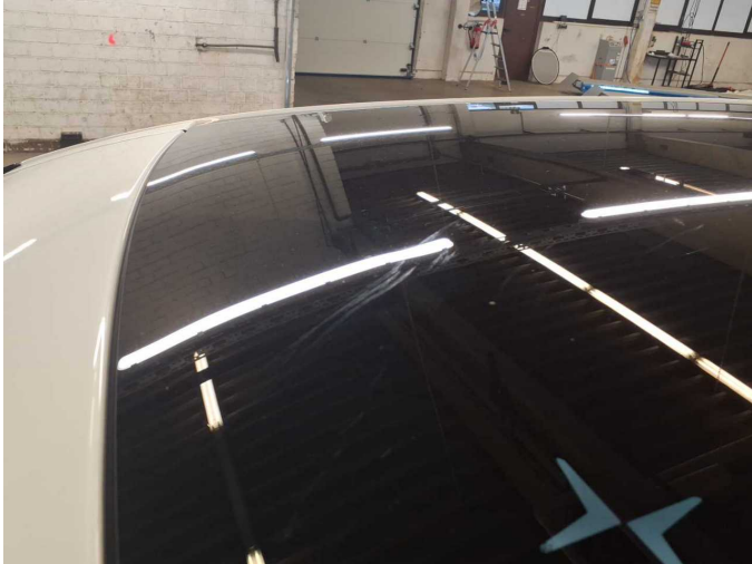
Damage 6: Roof: Sun roof / glass - Scratch(es) - Loss in value
