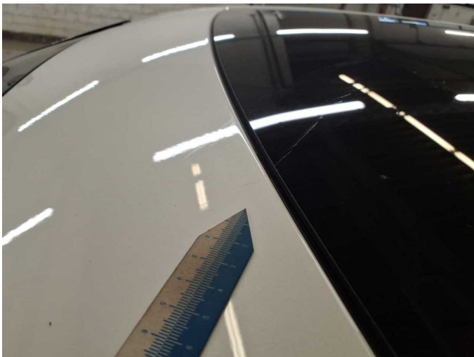
Damage 7: Roof: Roof - Scratch(es) - Paint
