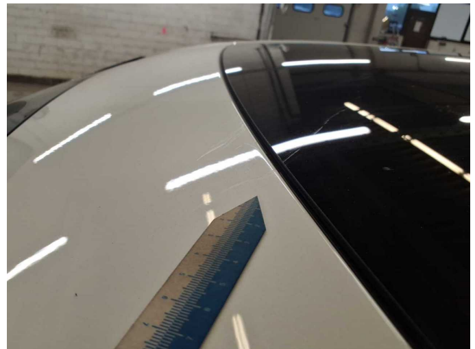
Damage 7: Roof: Roof - Scratch(es) - Paint
