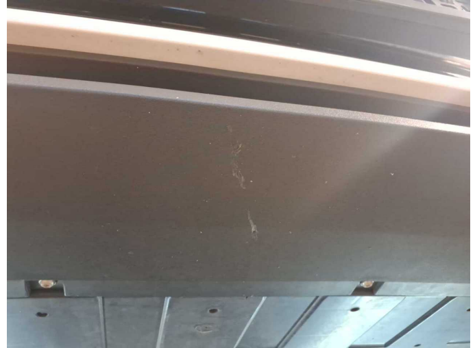
Damage 1: Front bumper: Spoiler - Scratch(es) - Replace
