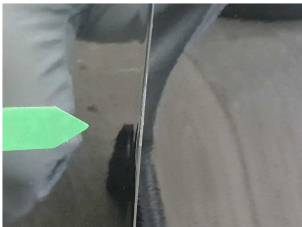
Beschädigung #4: Tür vorn links: Tür - Kratzer - Smart Repair
