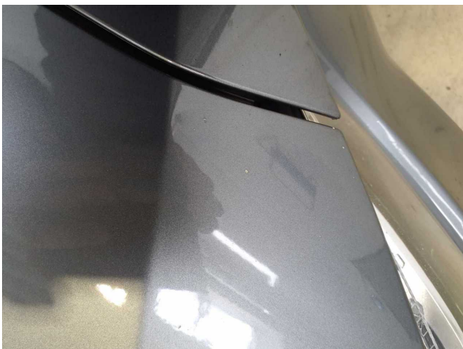
Damage 7: Bonnet: Bonnet - Dent / paintcoat damage - Loss in value
