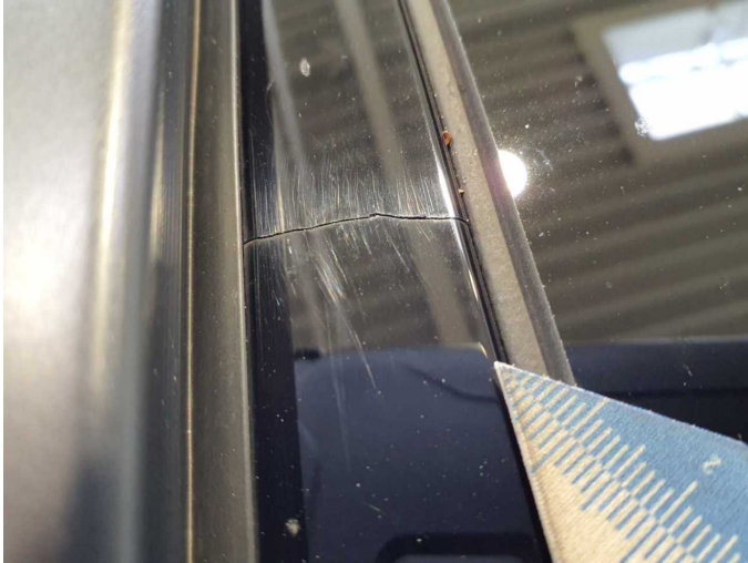
Damage 4: Roof: Cowl - right side - Broken / torn - Replace
