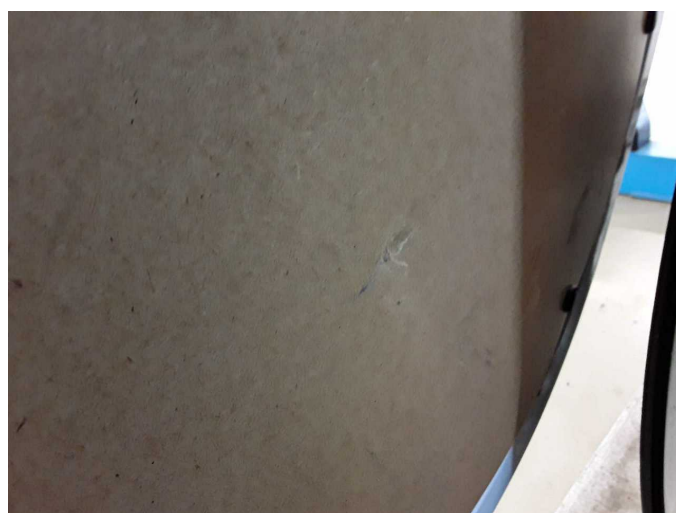
Damage 3: Sliding door, right: Trim hard fibre - lower - Broken / torn - Replace
