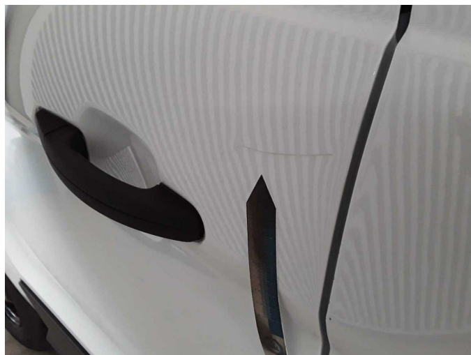
Damage 4: Sliding door, right: Sliding door - Dent / paintcoat damage - Smart repair
