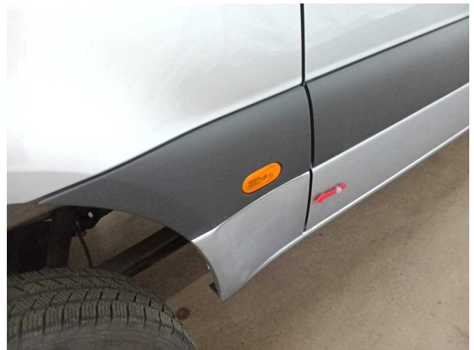
Damage 3: Side panel - rear right side: Side panel - Unprofessionally repaired - Repair and paint
