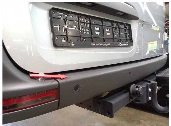
Damage 2: Rear bumper: Rear bumper - Scratched - Replace
