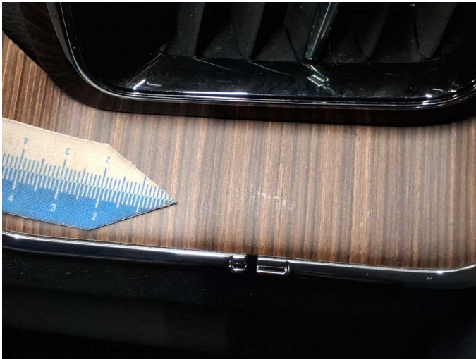
Wear and tear 3: Trim / covers: Brightware / decorative strip - Scratch(es) - No deduction
