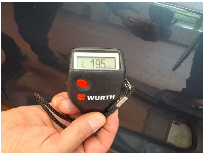
Repainting 2: Door - front left side
