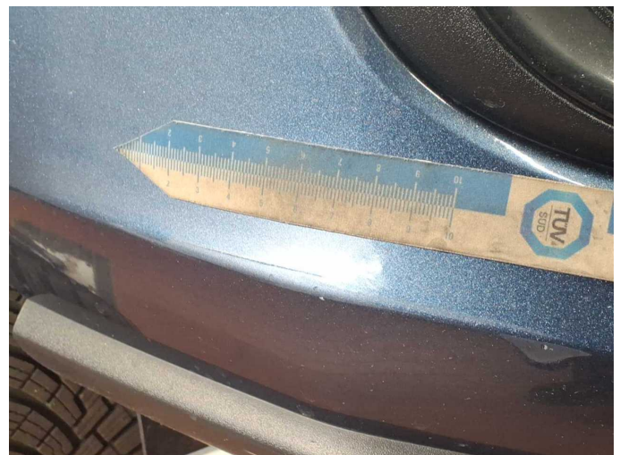
Damage 7: Front bumper: Front bumper (Lackläufer, Lackeinschlüsse) - Unprofessionally repaired - Repair and paint
