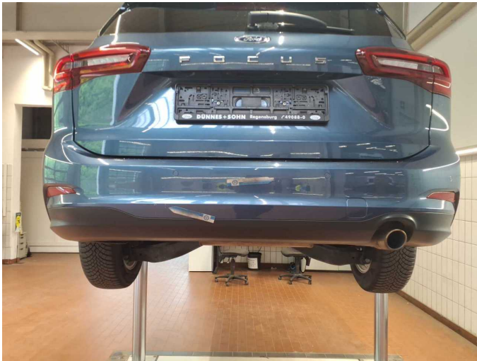
Damage 6: Rear bumper: Rear bumper - Scratch(es) - Paint
