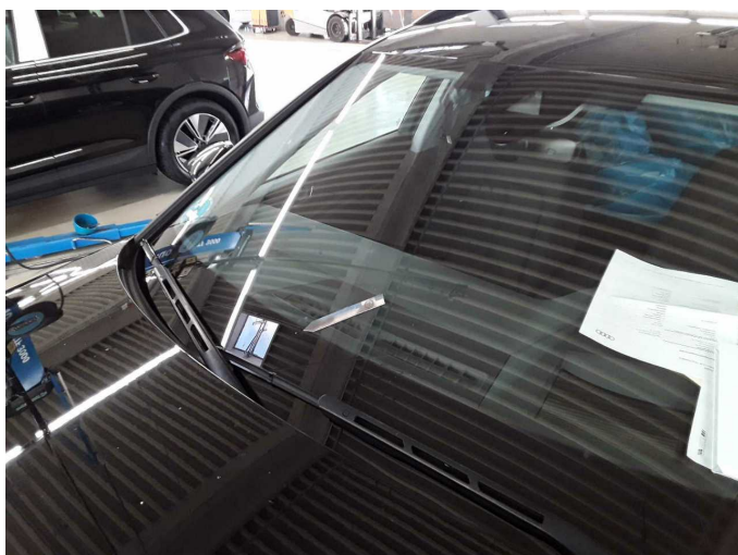
Damage 1: Vehicle glazing: Windscreen with lane departure assistant - Stone chips - repair according to calculation
