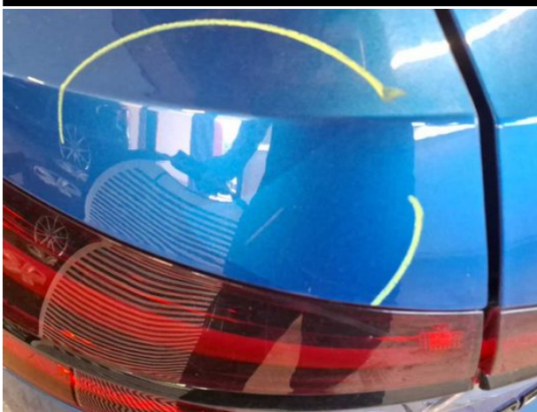
Damage #6: Side panel - rear left side: Side panel - Dent / paintcoat damage - Smart repair
