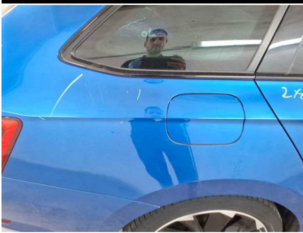
Damage #16: Side panel - rear right side: Side panel - Scratched - Repair and paint
