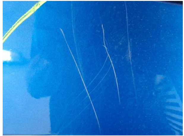
Damage #16: Side panel - rear right side: Side panel - Scratched - Repair and paint
