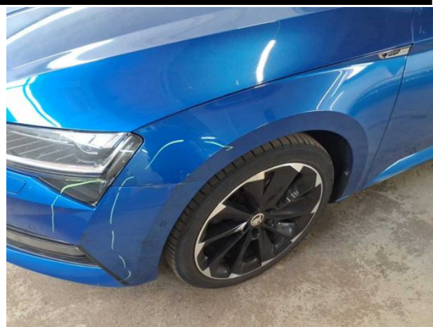
Damage #10: Mudguard - left side: Mudguard - left side - Scratched - Repair and paint
