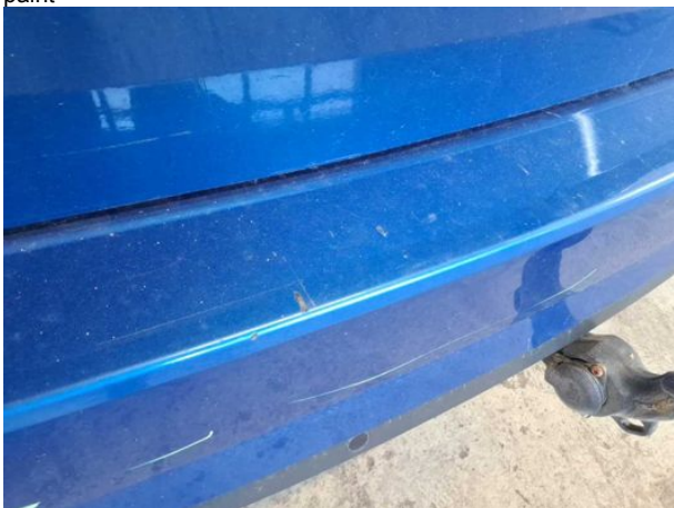
Damage #13: Rear bumper: Rear bumper - Scratched - Repair and paint
