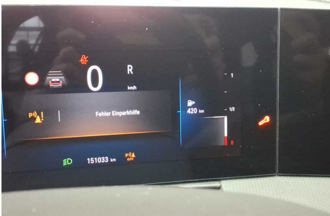
Damage 6: Instrument panel: Indicator light (Parkhilfe) - on - Perform diagnosis
