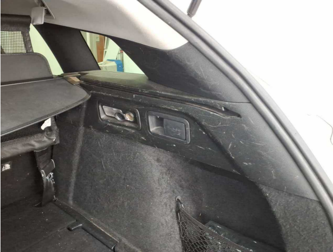
Damage 7: Interior: Interior - Scratch(es) - Loss in value
