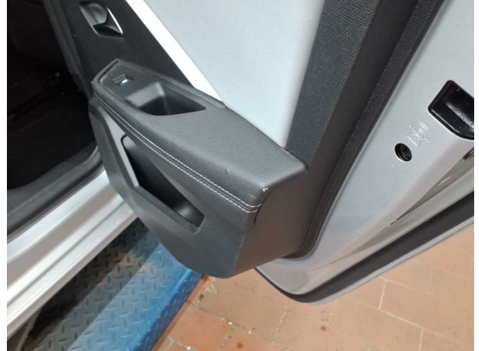
Damage 2: Trim / covers: Door trim - rear right side - Scratch(es) - Loss in value
