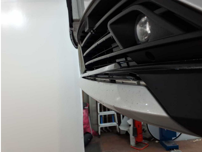
Damage 1: Trim / covers: Brightware / decorative strip - Loose - Repair
