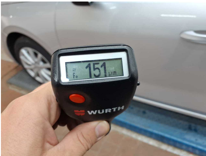
Repainting 1: Side panel - rear left side, Door - rear right side
