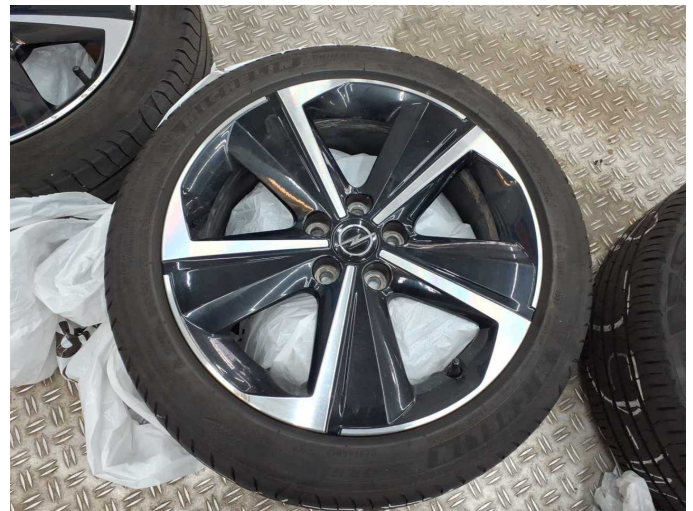
Damage 8: 2nd wheel set: 2 alloy rims - Scratch(es) - Loss in value
