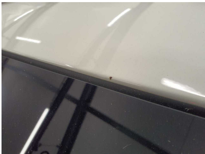
Damage 9: Roof: Roof (Korrosion) - Stone chips - Repair and paint
