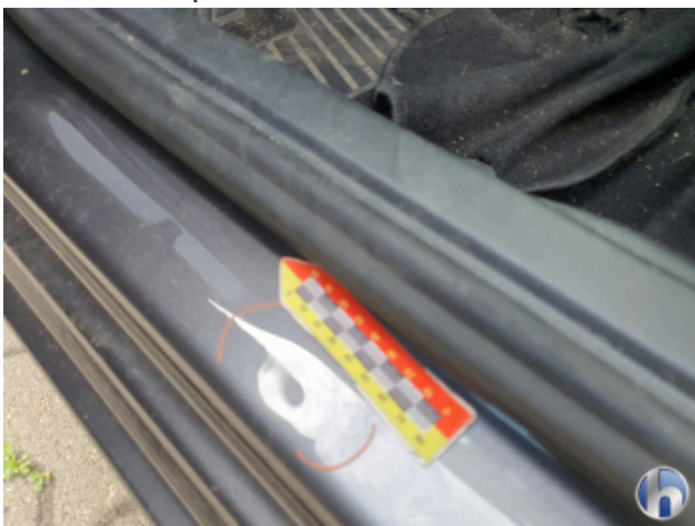
2. Türeinstieg Vorne - Links 1 Delle - Smart Repair
