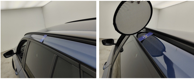
Roof // Smart Repair Medium-dent
