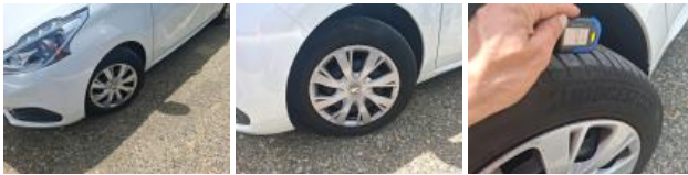
Tyre RL, Out of tolerance, Replace
