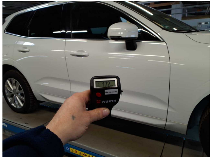
Repainting 1: Door - front right side
