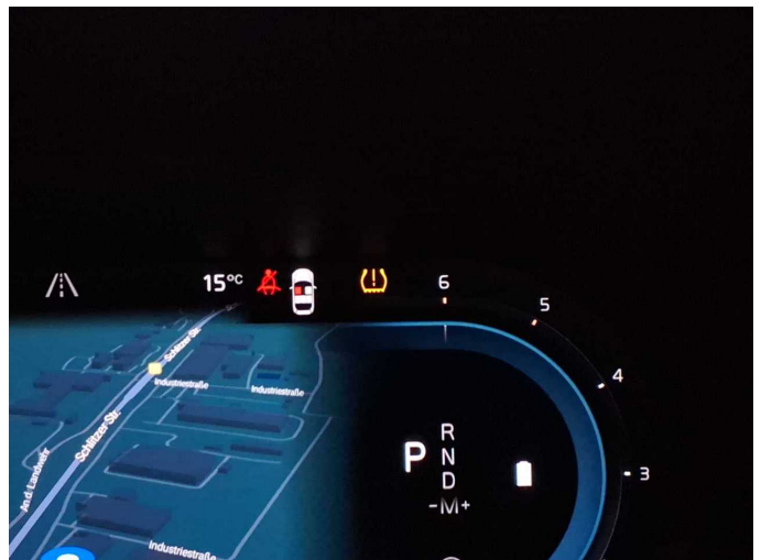
Damage 2: Wheel / tyres: Pressure sensor (Reifendruck) - Functional / admissibility - Perform diagnosis
