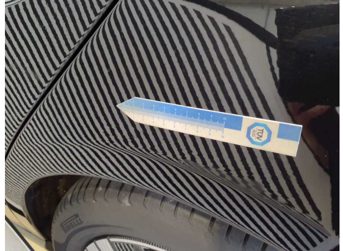
Damage 6: Side panel - rear left side: Side panel (Wellig und Spachtelmasse eingefallen) - Unprofessionally repaired - Repair and paint
