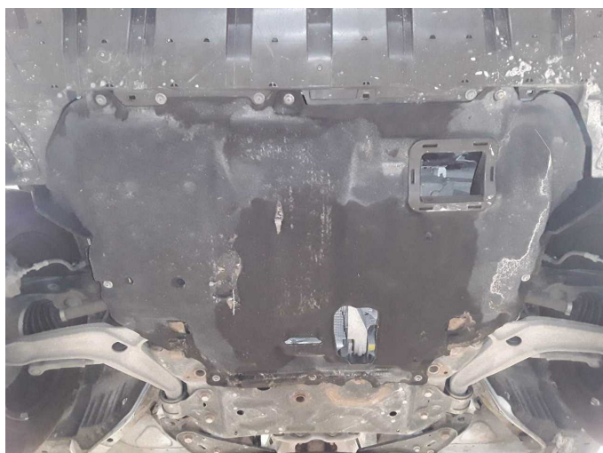
Damage 6: Body: Underbody panelling (Motor/Getriebe) - Leaking - Perform diagnosis
