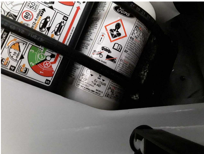
Damage 2: Equipment: Tirefit filler - Due - Replace
