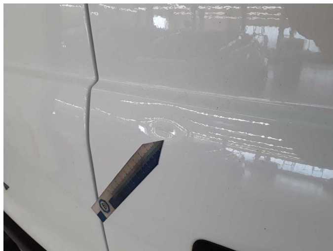
Damage 5: Boot lid / rear door: Rear door - right side - dent(s) - Smart repair
