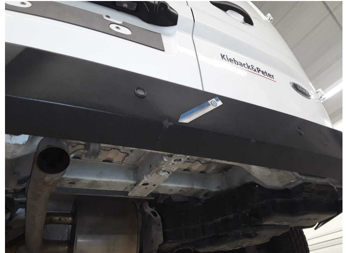
Damage 8: Rear bumper: Rear bumper (unpainted) - Scratched - Replace
