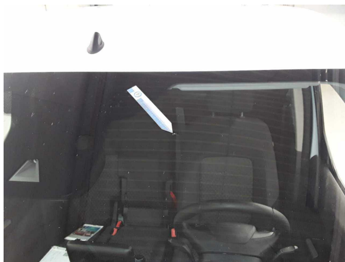
Damage 11: Vehicle glazing: Windscreen - Stone chips - Replace
