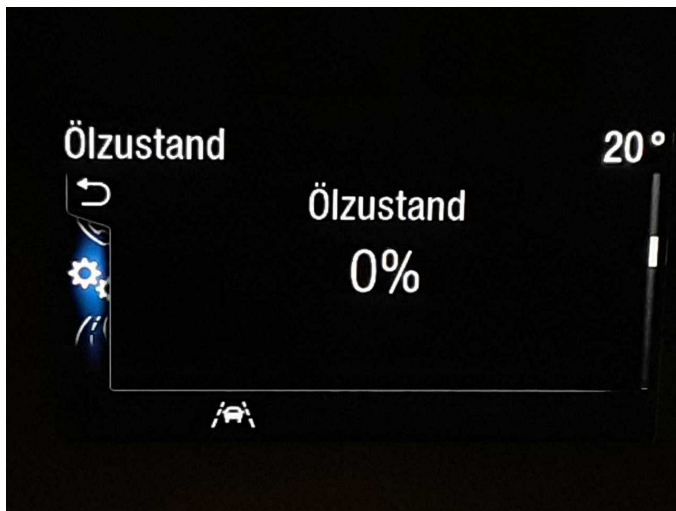
Damage 9: Misc.: Inspection / maintenance - Due - Perform
