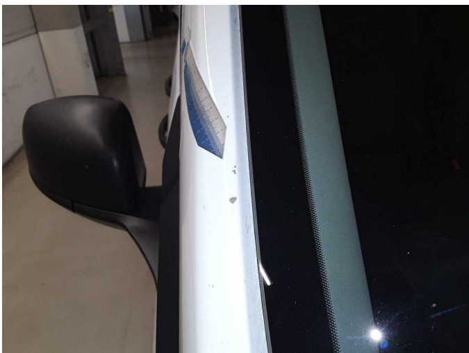
Damage 3: Roof: Roof rail - right side - Stone chips - Smart repair
