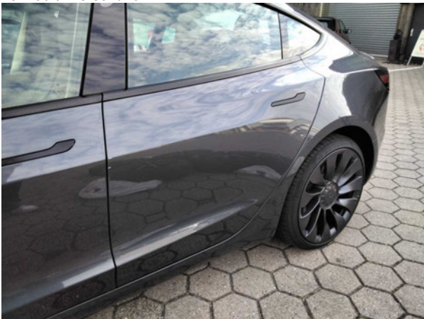
Beschädigung #2: Tür hinten links: Tür - Kratzer - Smart Repair
