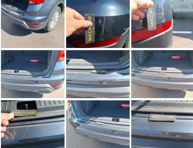
Rear window, Scratch(es), Replace
