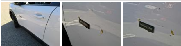
Wing trim FL, Scratch(es), Replace
