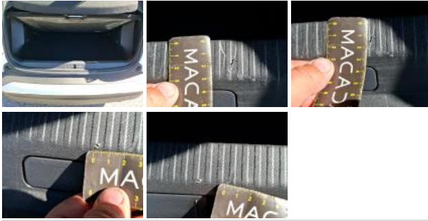
Boot lid covering R, Scratch(es), Replace
