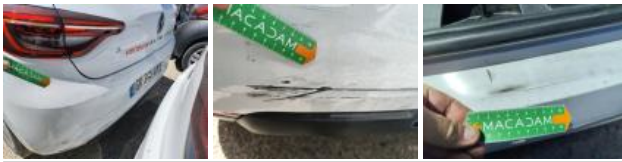
Tailgate / Boot, Dent(s), Repair and paint (complete)
