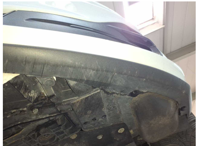
Damage 3: Front bumper: Spoiler - Scratched - Replace
