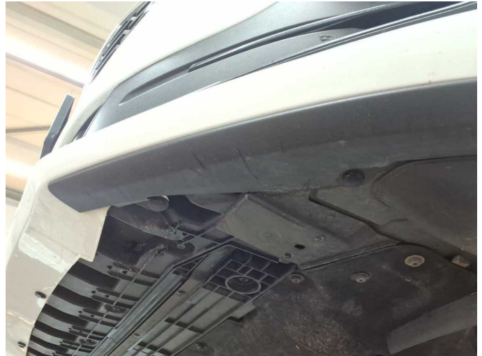
Damage 3: Front bumper: Spoiler - Scratched - Replace
