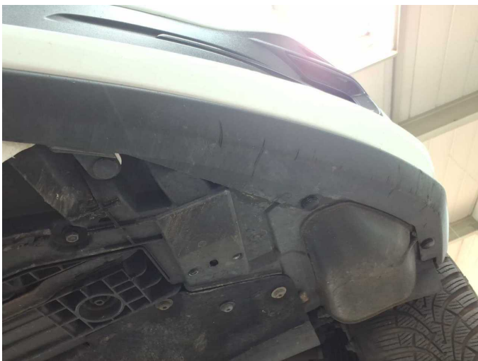
Damage 3: Front bumper: Spoiler - Scratched - Replace
