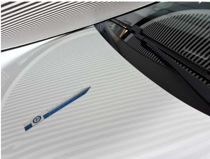
Damage 1: Bonnet: Bonnet - dent(s) - Smooth repair work
