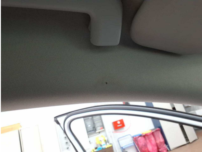
Damage 2: Trim / covers: Roof lining - Holes - Smart repair
