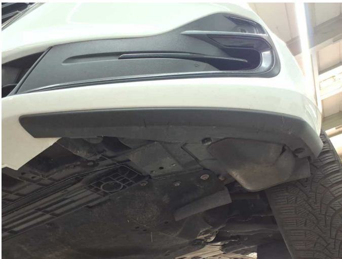
Damage 3: Front bumper: Spoiler - Scratched - Replace
