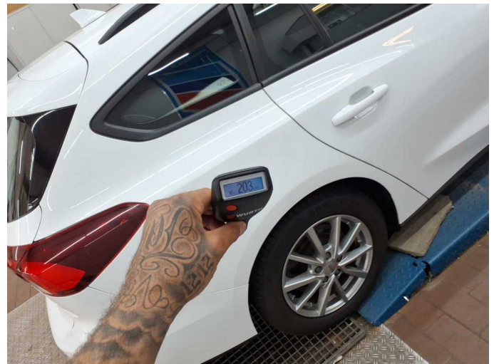
Repainting 1: Side panel - rear right side, Door - rear right side, Door - front right side
