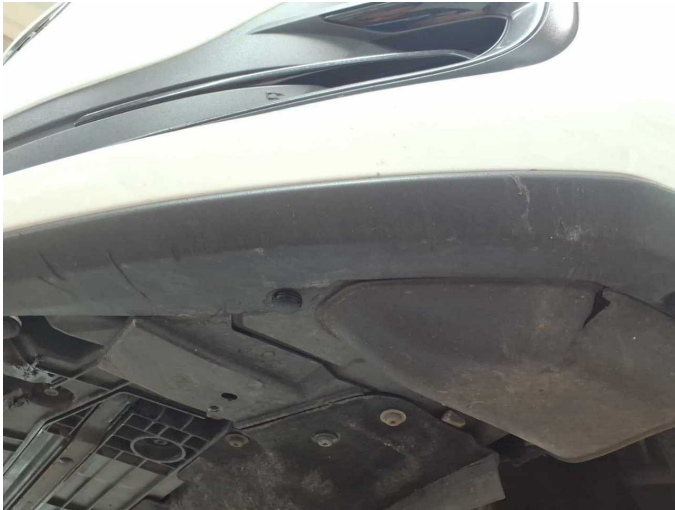
Damage 3: Front bumper: Spoiler - Scratched - Replace
