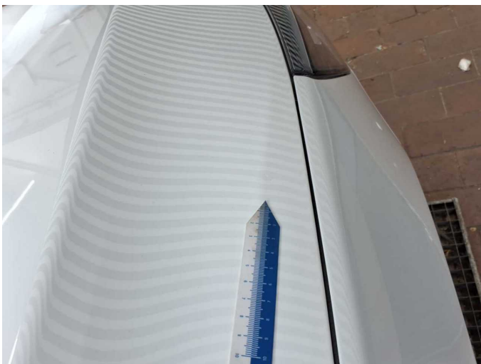
Damage 1: Bonnet: Bonnet - dent(s) - Smooth repair work
