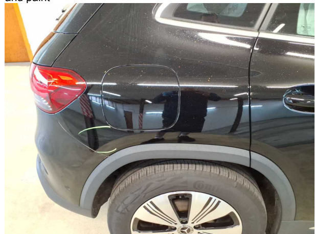
Damage #4: Side panel - rear right side: Side panel - Scratch... - Repair and paint
