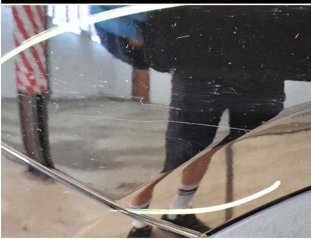
Damage #4: Side panel - rear right side: Side panel - Scratched - Repair and paint
