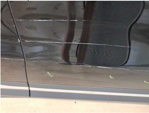
Damage #5: Door - front right side: Door - Scratched - Replace
