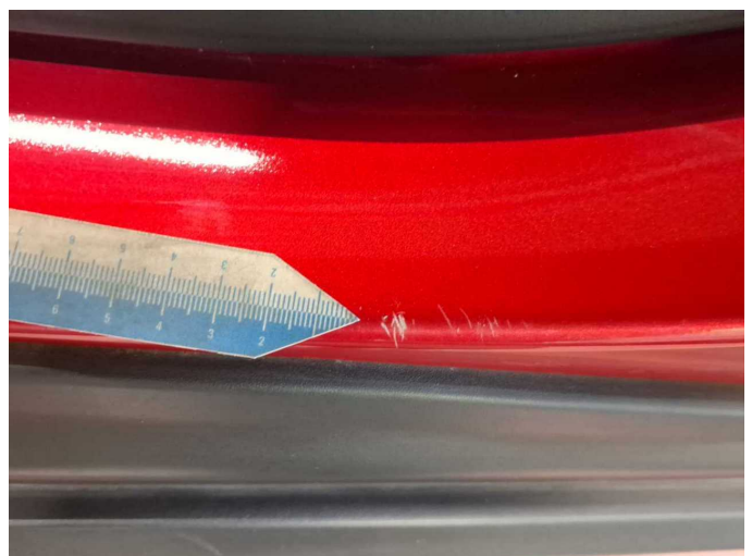
Damage 3: Sill - left side: Sill - Scratch(es) - Smart repair
