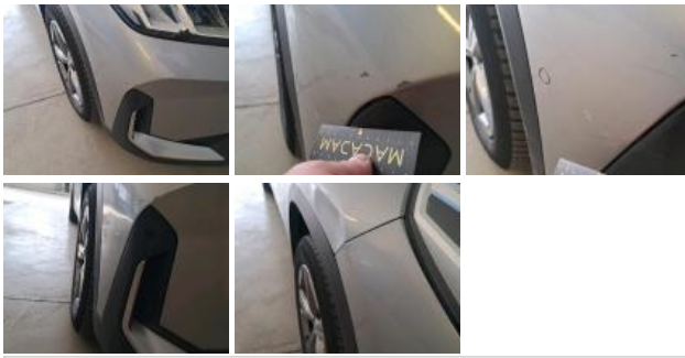
Door RL, Scratch(es), Repair and paint (complete)
