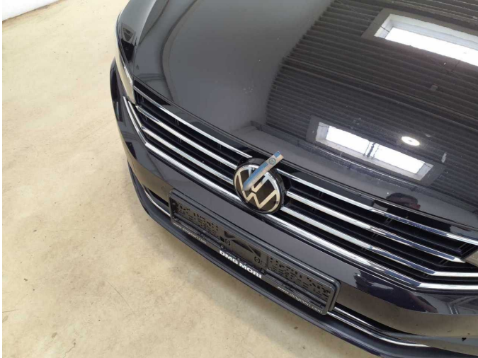
Damage 11: Front structure: Emblem - Broken / torn - Replace
