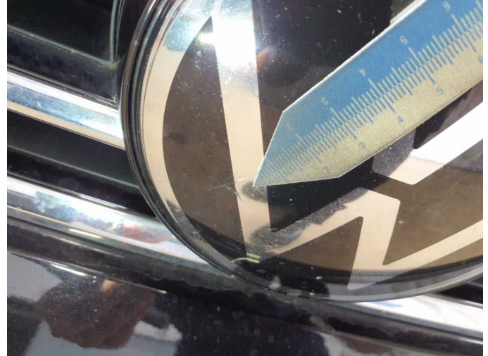
Damage 11: Front structure: Emblem - Broken / torn - Replace
