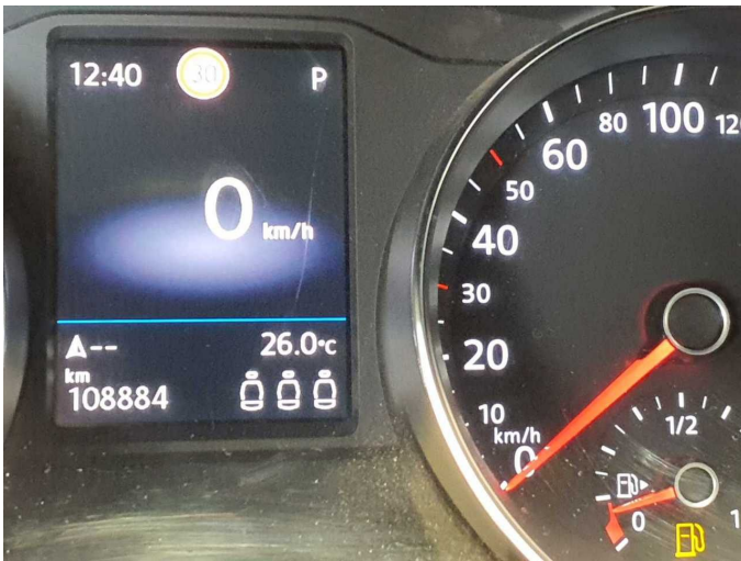
Damage 12: Instrument panel: Instrument cluster - Scratch(es) - Loss in value
