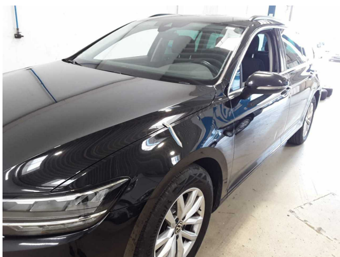
Damage 3: Mudguard - left side: Mudguard - left side - Paint defect - Repair and paint
