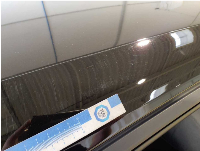
Damage 5: Roof: Roof rail - right side - Scratch(es) - Paint
