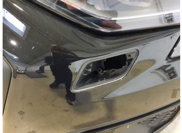
Damage 1: Headlight: Headlight cleaning nozzle - left side (Waschwasserdüse) - Missing - Replace
