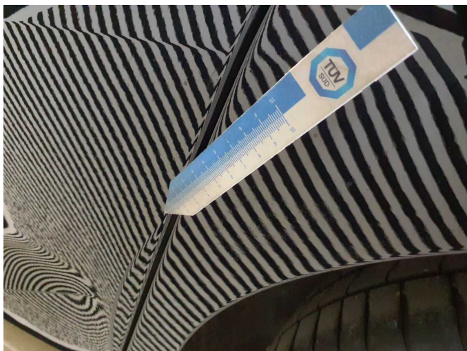
Damage 7: Side panel - rear left side: Side panel (Spachtelmasse eingefallen) - Unprofessionally repaired - Repair and paint
