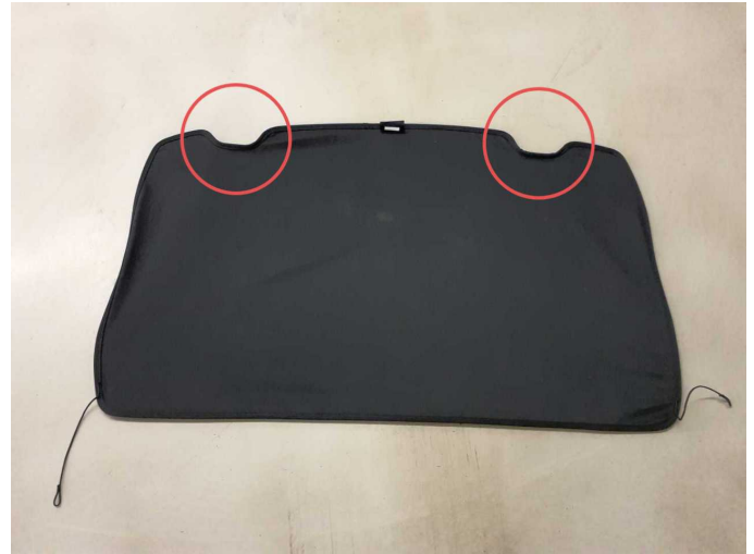
Missing part 1: Interior: Boot cover / roller cover (Halterungen) - Missing - Replace
