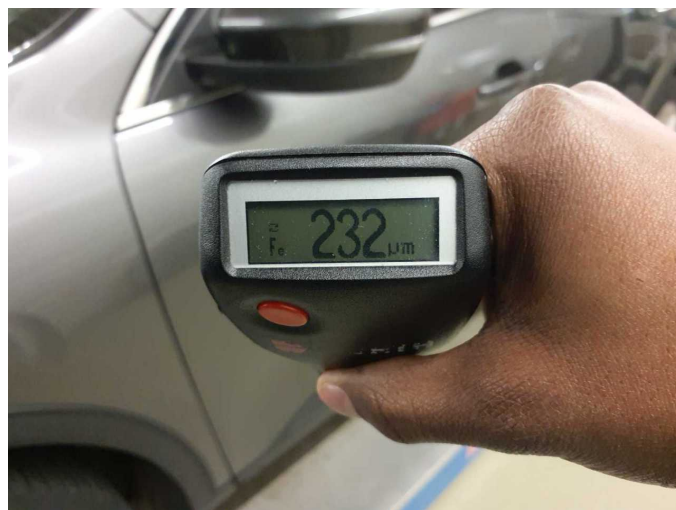
Repainting 3: Door - front left side
