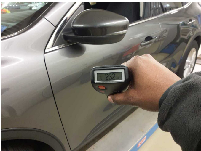
Repainting 3: Door - front left side
