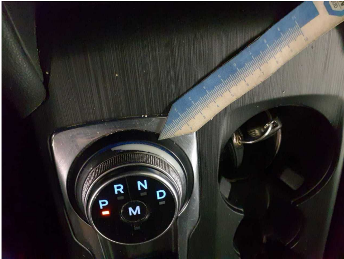
Wear and tear 2: Gearbox: Gear knob (Chrome löst sich) - Loose - No deduction
