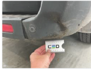
4 - Bumper corner RR - Deformed / Strained
