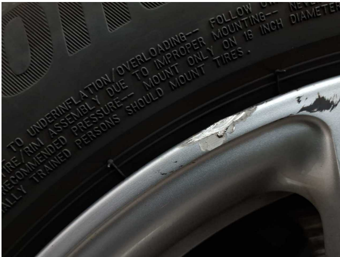
Wear and tear 3: Wheel / tyres: Alloy rim - front right side - Scratched - No deduction
