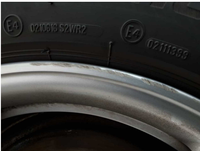
Wear and tear 4: Wheel / tyres: Alloy rim - rear right side - Scratched - No deduction
