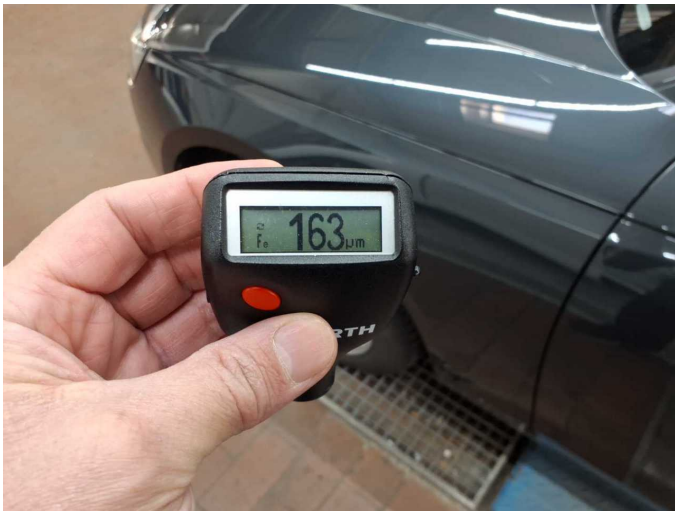
Repainting 1: Mudguard - left side, Bonnet, Side panel - rear right side, Door - rear left side, Door - front left side
