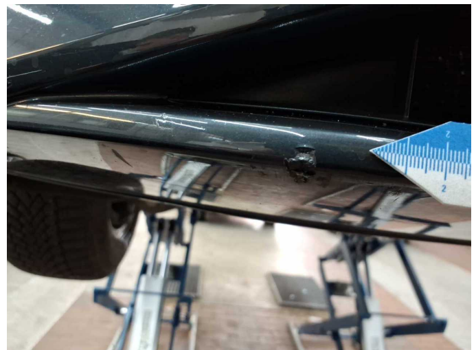
Damage 4: Front bumper: Front bumper - Scratched - Paint
