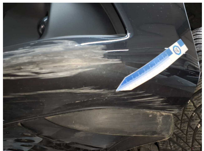
Damage 4: Front bumper: Front bumper - Scratched - Paint
