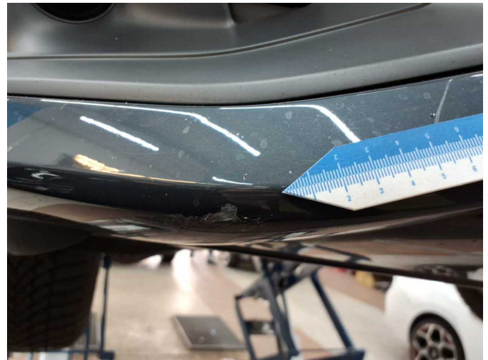
Damage 4: Front bumper: Front bumper - Scratched - Paint
