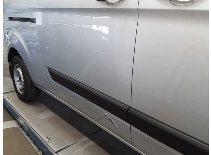
Damage 2: Sliding door, right: Sliding door - Deformed - Smart repair
