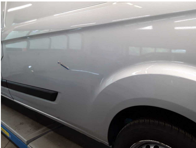
Damage 4: Side panel - rear right side: Side panel - Scratched - Paint
