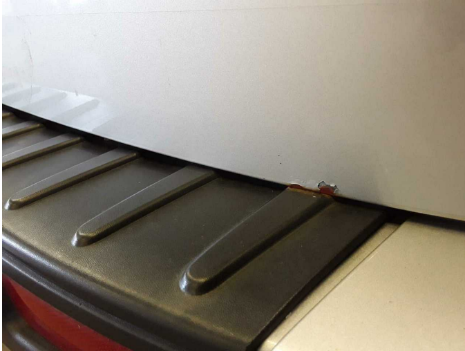
Damage 1: Boot lid / rear door: Rear door - right side - Corrosion - Smart repair
