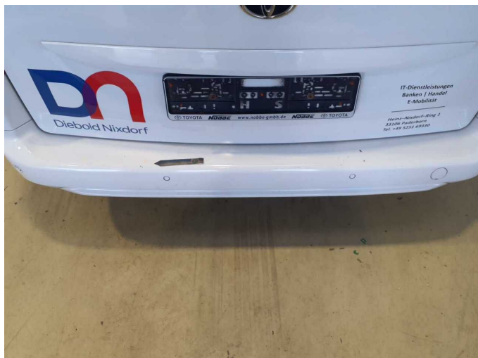
Damage 15: Rear bumper: Rear bumper - Scratch(es) - Paint
