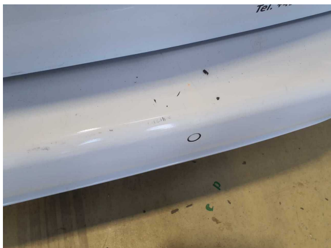
Damage 15: Rear bumper: Rear bumper - Scratch(es) - Paint
