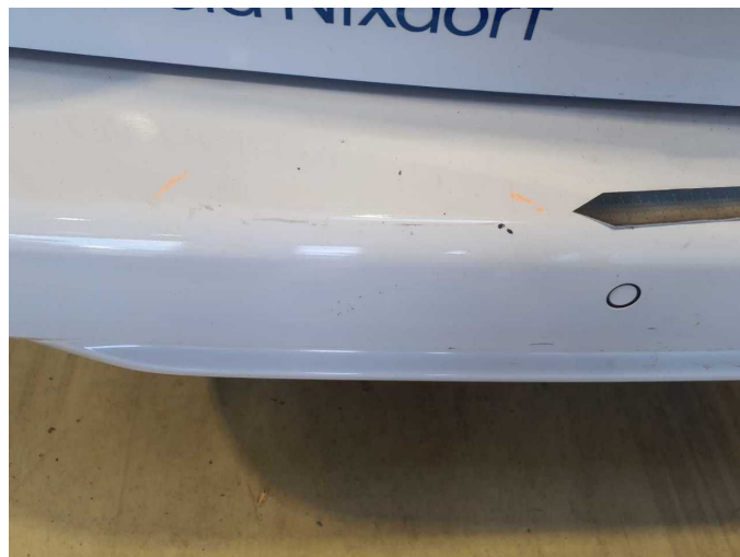
Damage 15: Rear bumper: Rear bumper - Scratch(es) - Paint
