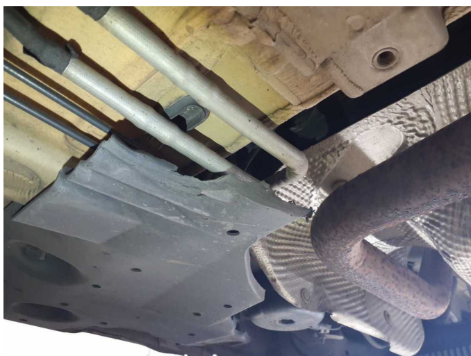
Damage 9: Body: Underbody panelling - Broken / torn - Replace
