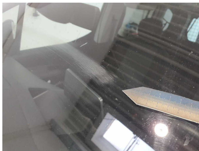
Damage 16: Vehicle glazing: Windscreen - Scratched - Replace
