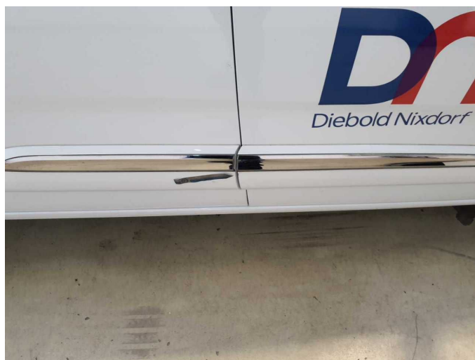
Damage 7: Door - front right side: Brightware - lower - Scratch(es) - Smart repair
