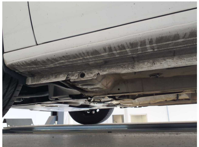
Damage 11: Sill - left side: Sill - Deformed - Smart repair
