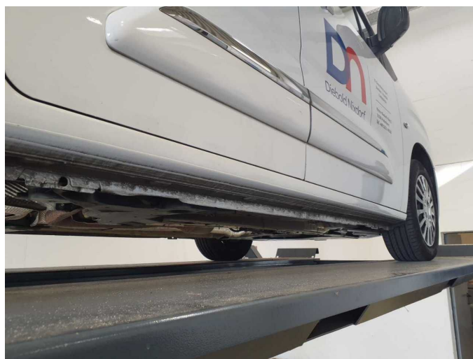
Damage 10: Sill - right side: Sill - Deformed - Smart repair
