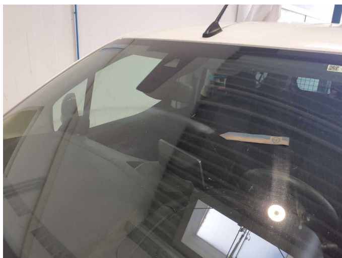
Damage 16: Vehicle glazing: Windscreen - Scratched - Replace
