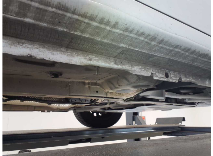
Damage 10: Sill - right side: Sill - Deformed - Smart repair
