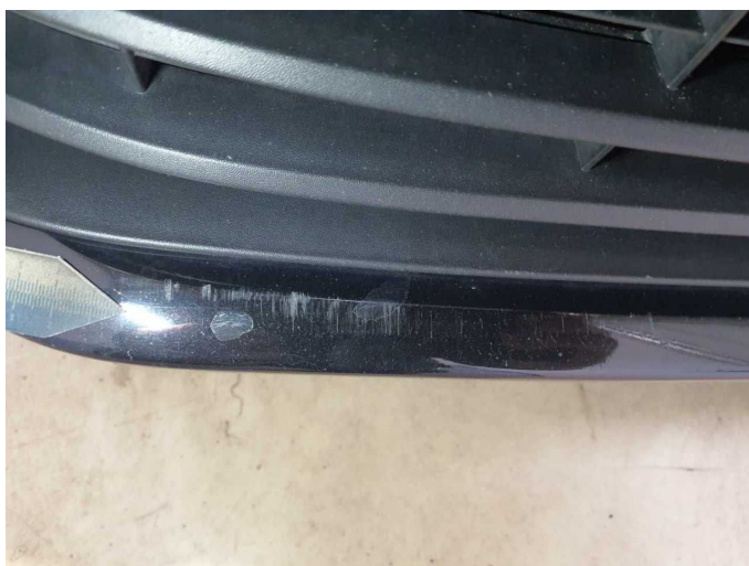
Damage 6: Front bumper: Spoiler - Scratch(es) - Smart repair
