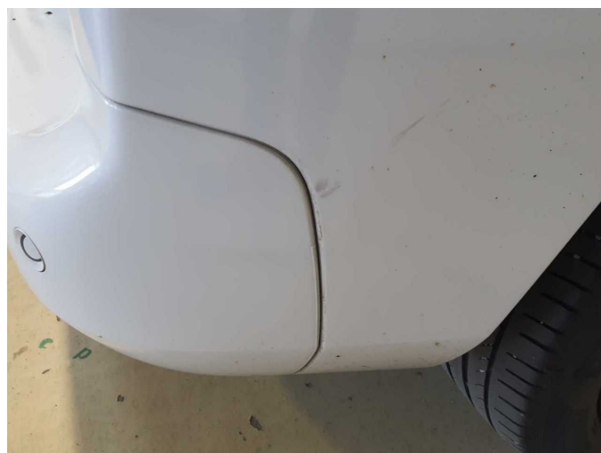
Damage 15: Rear bumper: Rear bumper - Scratch(es) - Paint
