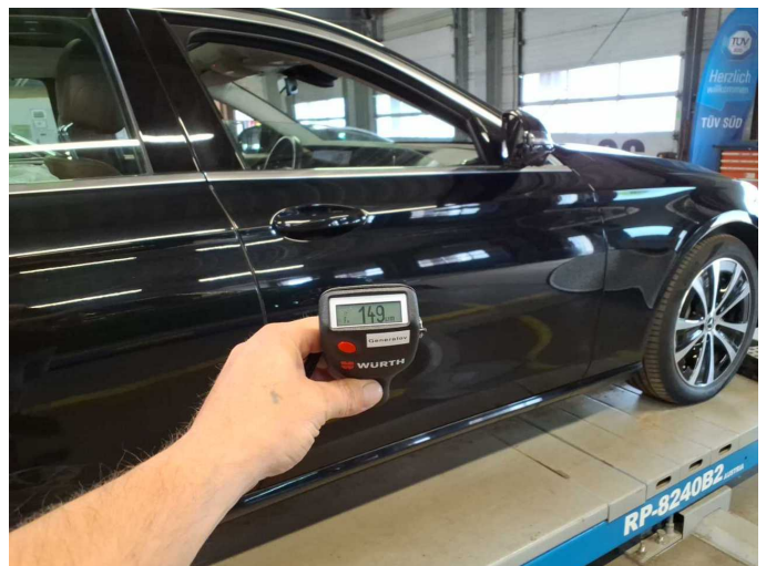
Repainting 3: Door - front right side
