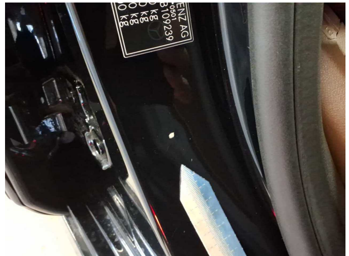
Damage 1: Body: B-pillar - right side - Dent / paintcoat damage - Smart repair
