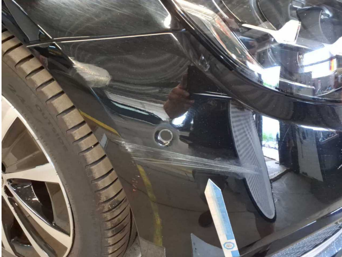
Damage 7: Front bumper: Front bumper - Scratched - Paint
