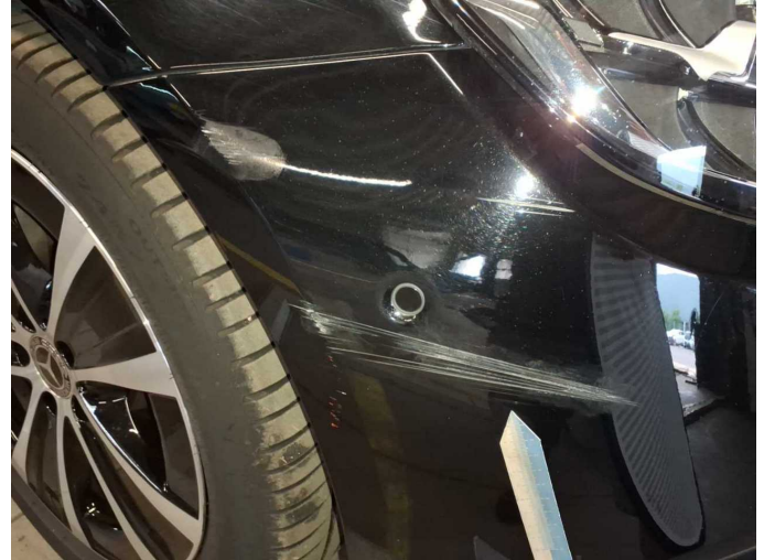
Damage 7: Front bumper: Front bumper - Scratched - Paint
