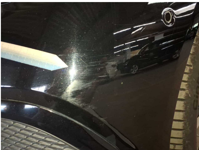
Damage 7: Front bumper: Front bumper - Scratched - Paint
