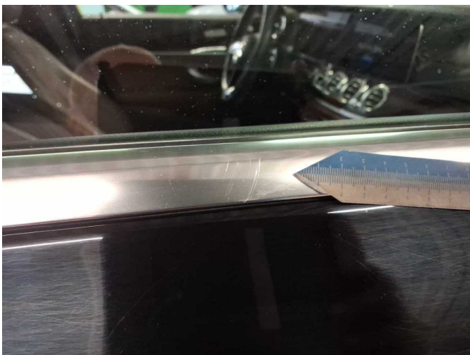
Damage 4: Door - front right side: Strip - outer - Scratch(es) - Replace
