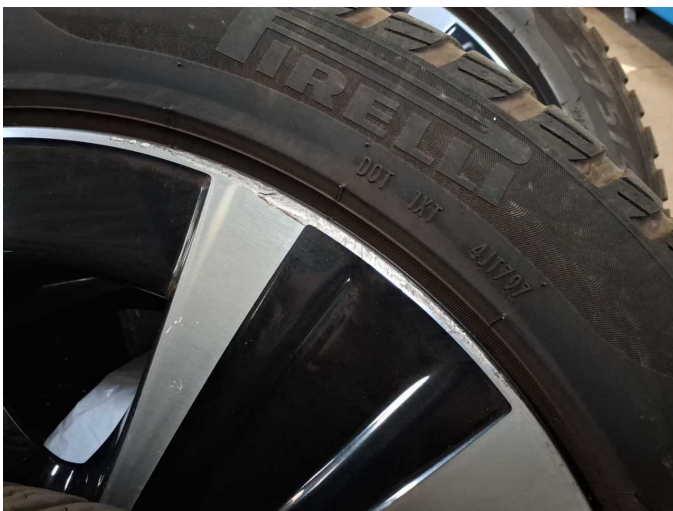
Wear and tear 2: 2nd wheel set: 2 alloy rims (Materialabtrag) - Scratched - No deduction
