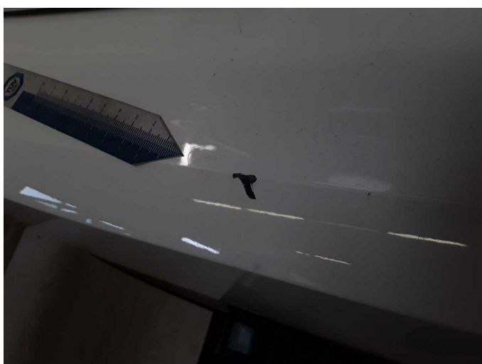
Damage 6: Rear bumper: Rear bumper - Scratch(es) - Paint
