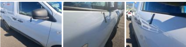
Door FR, Dent(s), Repair and paint (complete)
