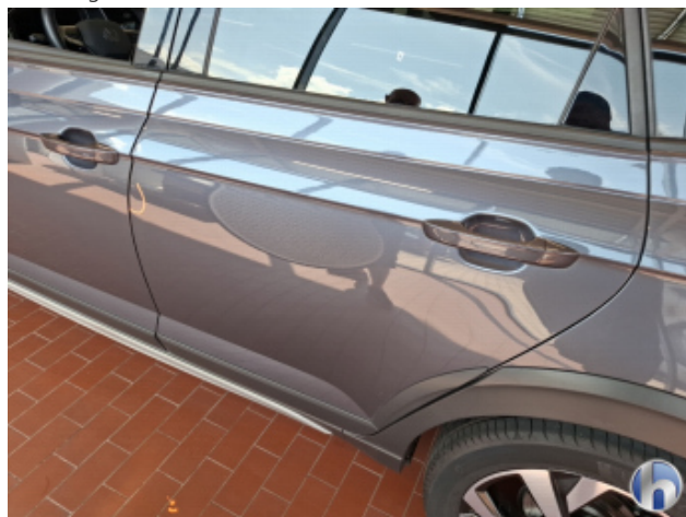
1. Tür Hinten - Links 1 Delle - Sanft Instandsetzen
