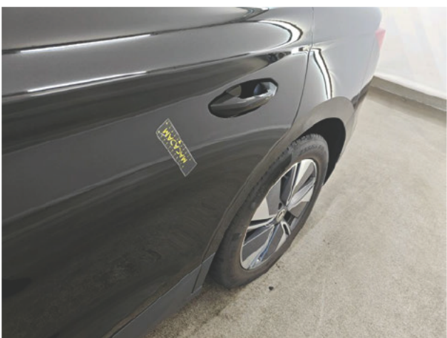
Door RL Bad repair Repair and paint (complete) Left
