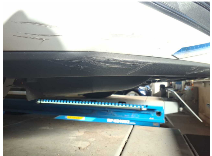
Damage 2: Front bumper: Spoiler - Scratched - Replace
