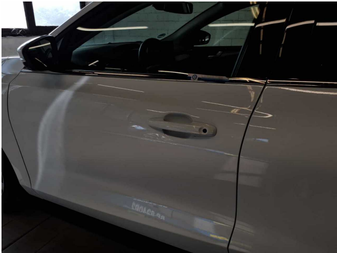
Damage 1: Door - front left side: Strip - outer - dent(s) - Loss in value
