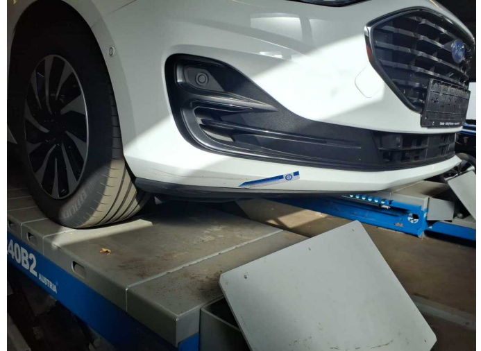
Damage 2: Front bumper: Spoiler - Scratched - Replace
