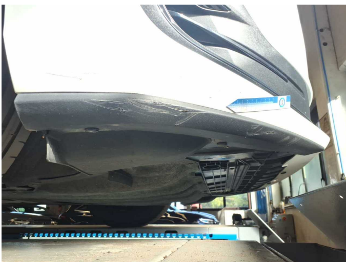
Damage 2: Front bumper: Spoiler - Scratched - Replace
