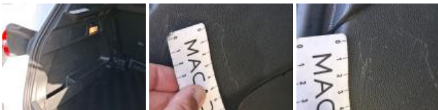
Internal boot lining L, Scratch(es), Repair/replace (lump sum)
