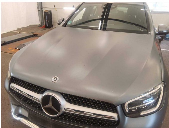
Damage 9: Bonnet: Bonnet - Dent / paintcoat damage - Repair and paint
