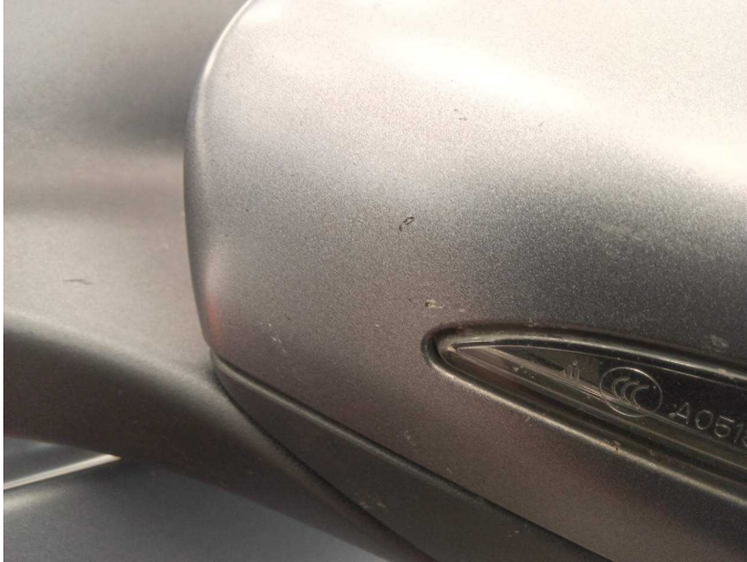
Damage 3: Wing mirror - left side: Cap - Scratch(es) - Replace
