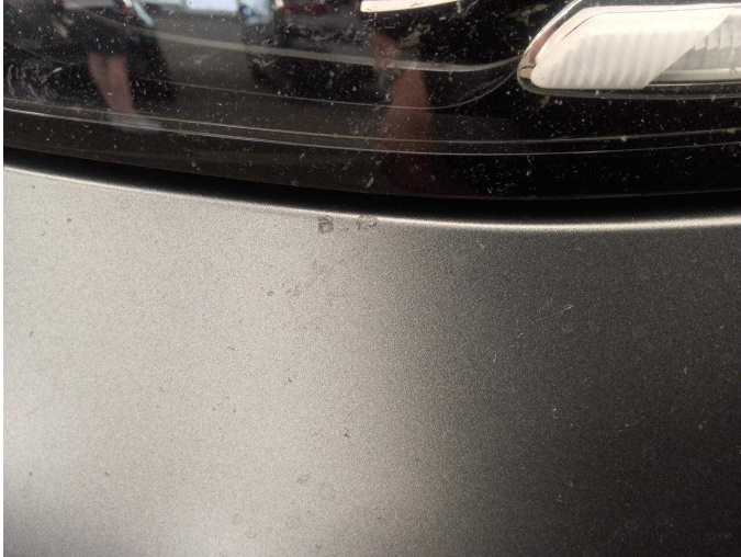
Damage 7: Front bumper: Front bumper (Sandstrahleffekt) - Stone chips - Paint
