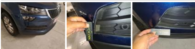
Bumper moulding F, Scratch(es), Replace
