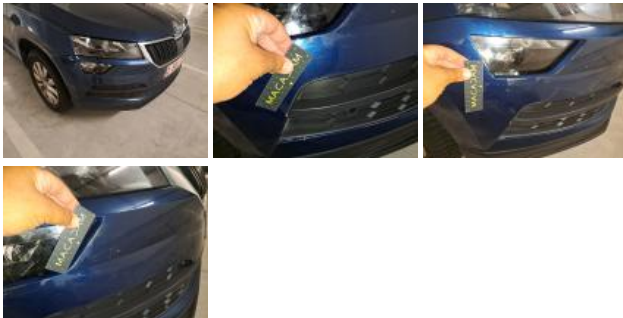
Bumper moulding F, Broken, Replace
