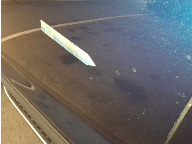
Damage 7: Door - front left side: Door - Scratch(es) - Paint
