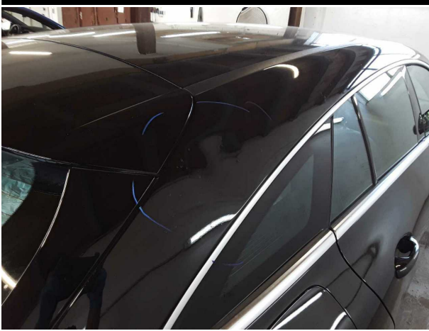
Damage #6: Roof: Roof rail - right side - dent(s) - Repair and paint
