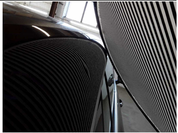
Damage #6: Roof: Roof rail - right side - dent(s) - Repair and paint
