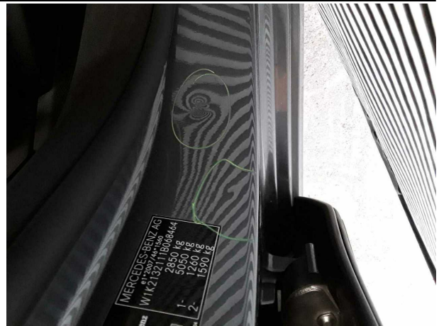
Damage #8: Sill - right side: Sill - Dent / paintcoat damage - Smooth repair work
