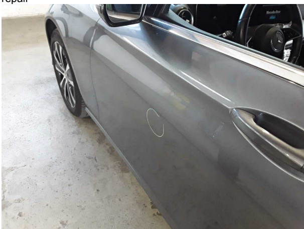
Damage #7: Door - front left side: Door - dent(s) - Smooth repair work
