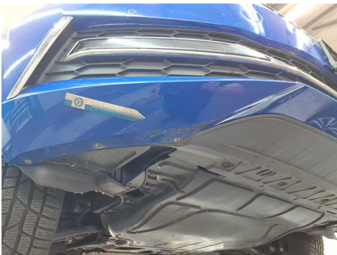
Damage 3: Front bumper: Front bumper - Scratch(es) - Loss in value
