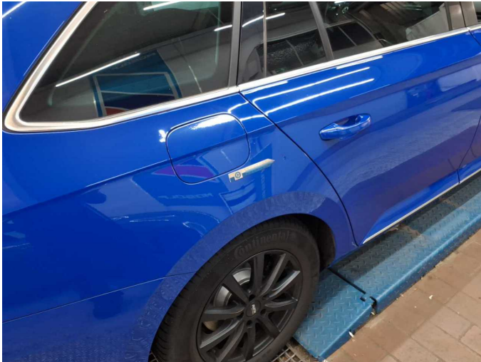
Damage 5: Side panel - rear right side: Side panel - Dent / paintcoat damage - Smart repair
