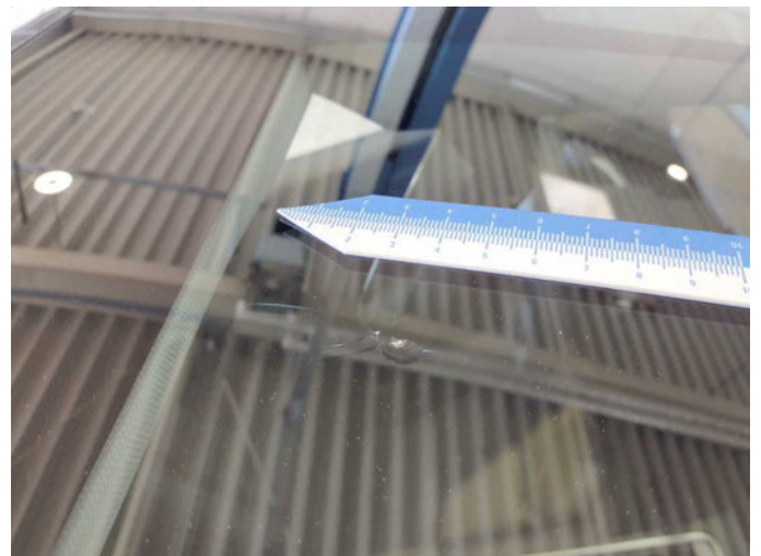
Damage 7: Vehicle glazing: Windscreen - Broken / torn - Replace
