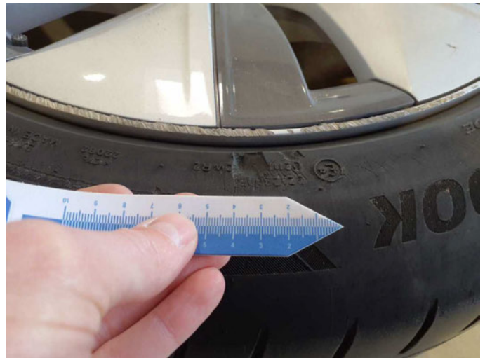
Damage 4: 2nd wheel set: 1 tyre - Scratched - Replace
