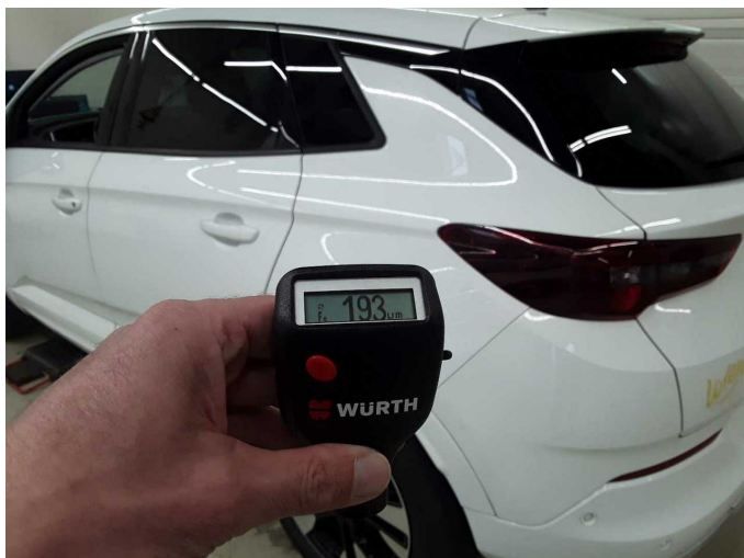
Side panel - rear left side: 193 µm
