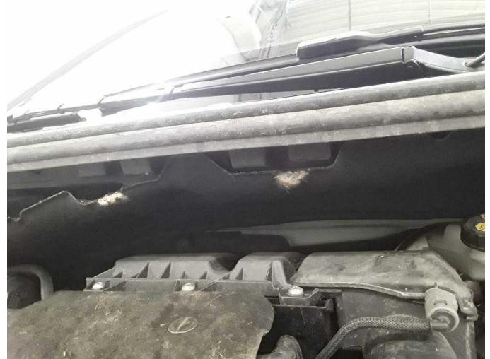
Damage 2: Body: Firewall trim (Mehrkosten möglich) - Damage caused by marten / rodent - Replace
